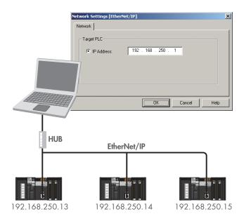
» Even if the IP address is not known, it is easy to connect by searching the PAC's on the EtherNet/IP network and selecting from a list.
