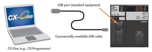
» A CJ2 CPU Unit on an EtherNet/IP Network Can Be Accessed Via USB, with No Need for Routing Tables.
