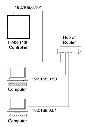
To connect to an HMS 1100 controller on a local network using HMS PC Access, under *Configure* >> *Network* enter the controller's IP address:
