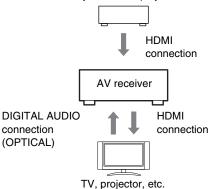
Connect the audio output from the TV to the OPTICAL IN 2 jack of the AV receiver using an optical digital cable.
