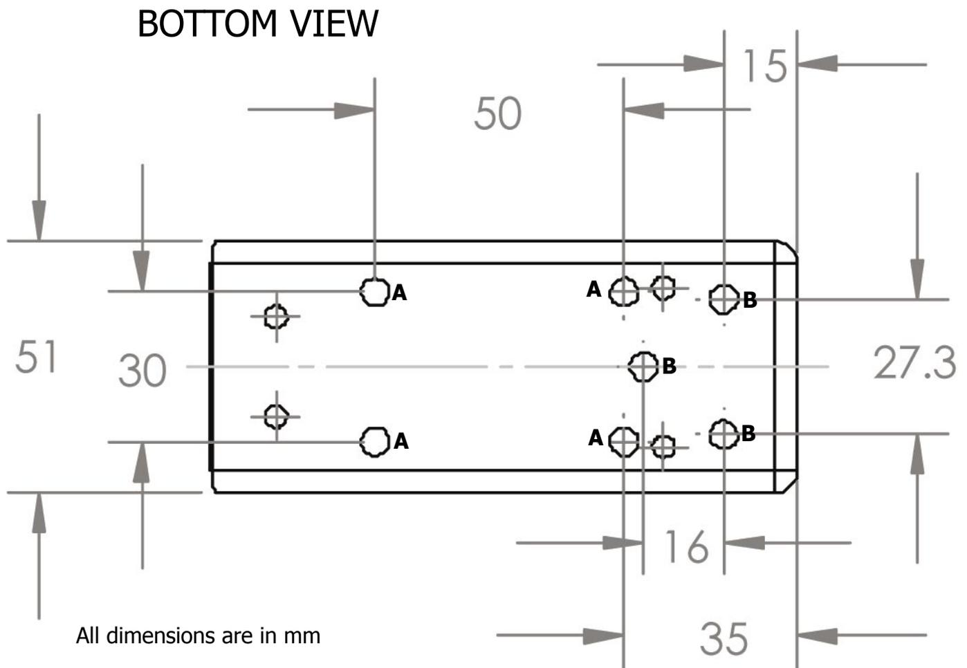
A = Four A type mounting holes represent the Opticon standard bracket.
