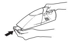
The crevice tool is stored on the back bottom of the vacuum. To remove tool, simply slide out of slot. Replace tool when finished to prevent loss.
