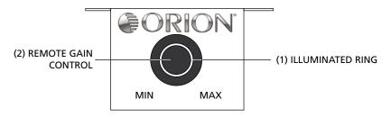
The front panel of the RGC2 consists of:
