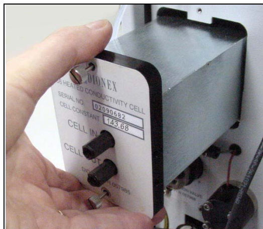
Figure 5-19. Removing the Cell Assembly
