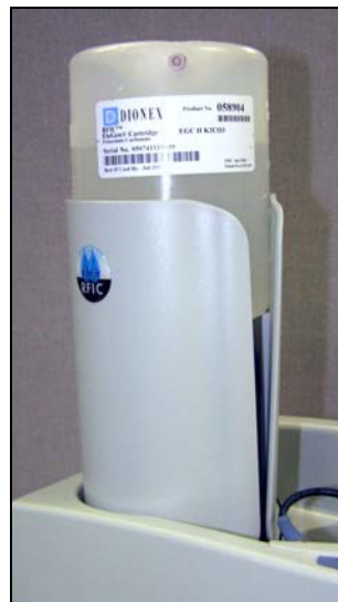
Figure 5-52. EluGen Cartridge Installed in the Holder
