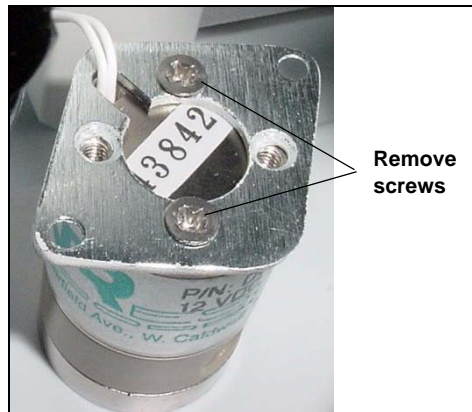
Figure 5-28. Removing the Eluent Valve Mounting Plate
