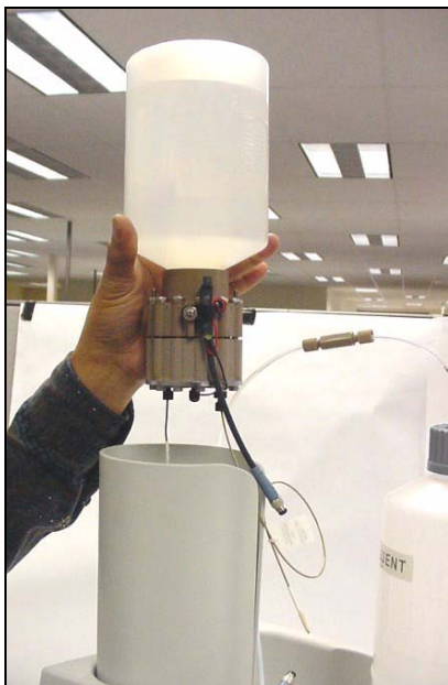
Figure 5-42. Installing the EluGen Cartridge in the Holder
