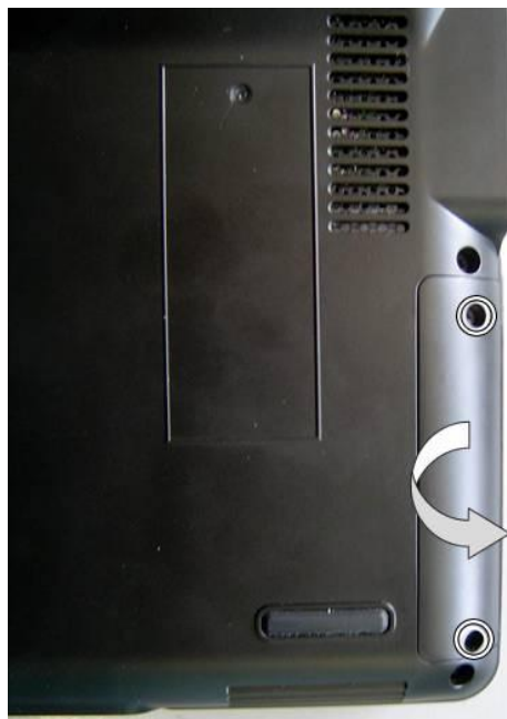
Fig. 2 Removing the hard disk drive cover.
