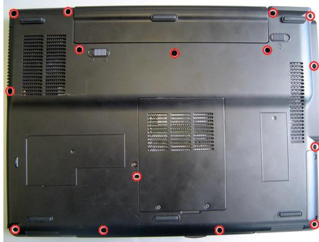
Fig. 15 Removing the bottom cover screws.
