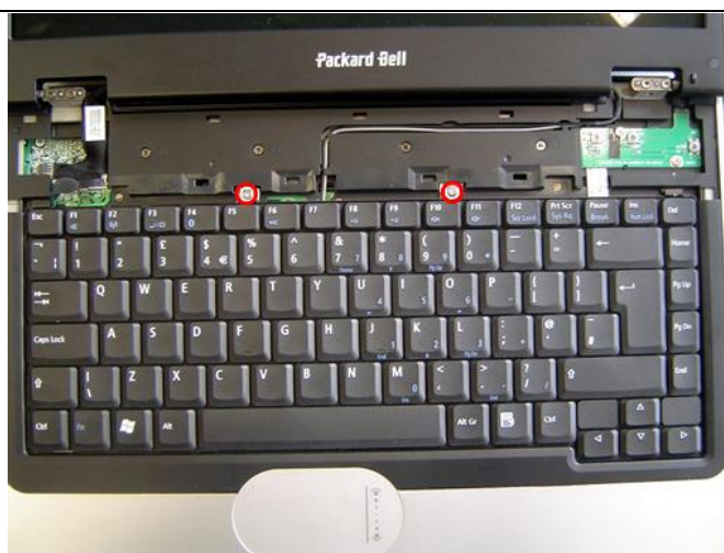
Fig. 13 Releasing the keyboard.
