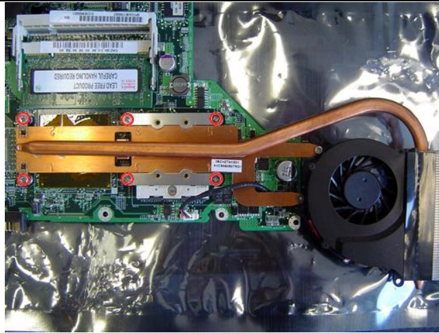
Fig. 22 Removing the heat sink.
