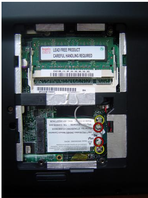
Fig. 9 Removing the WLAN card.
