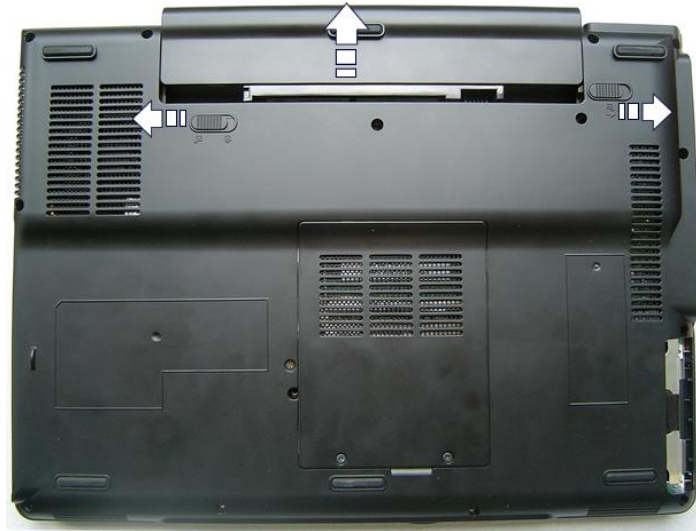
Fig. 1 Removing the battery.
