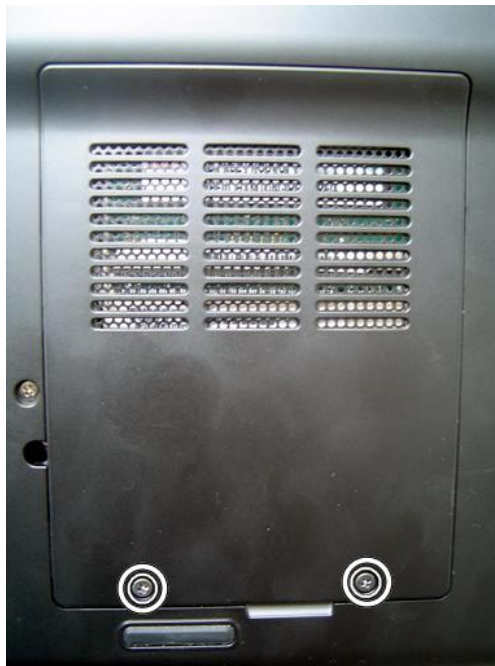
Fig. 7 Removing the memory slot cover.
