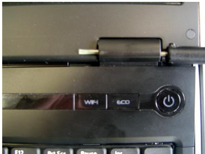
Fig. 12 Releasing the keyboard cover.
