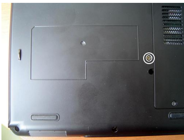
Fig. 5 Releasing the optical disk drive.
