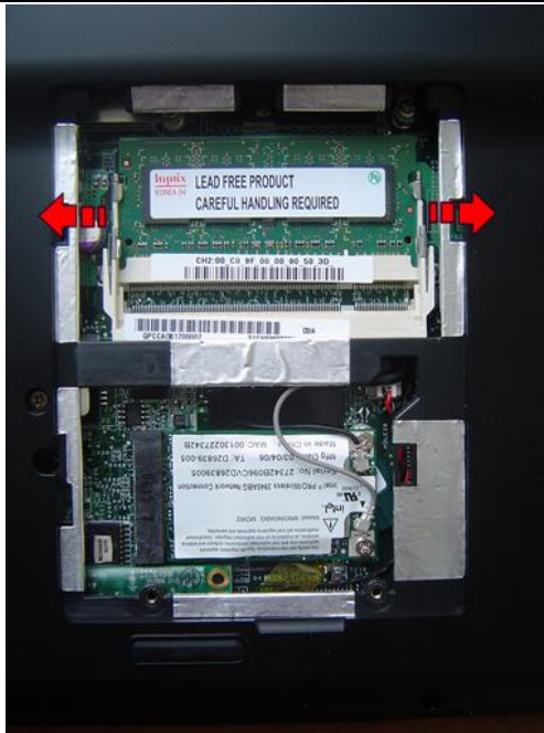
Fig. 8 Removing the memory module.
