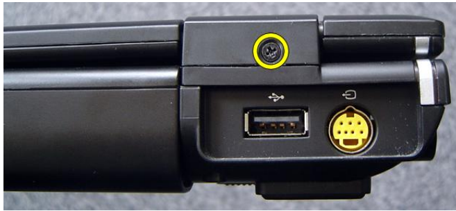
Fig. 11 Right keyboard back screw.
