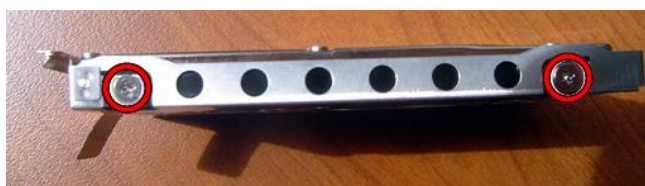
Fig. 4 Unscrewing the hard disk drive shield screws.
