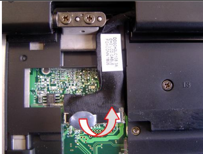
Fig. 17 Removing the LCD module.
