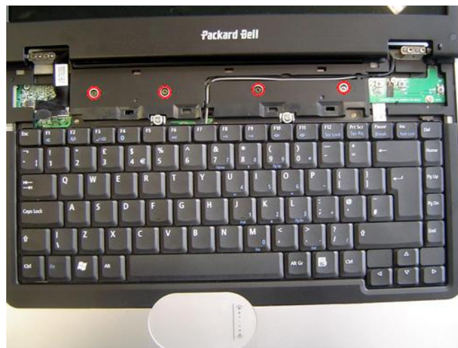
Fig. 16 Releasing the top cover.
