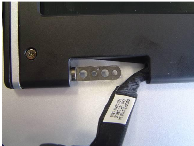
Fig. 18 Removing the LCD cover screws.
