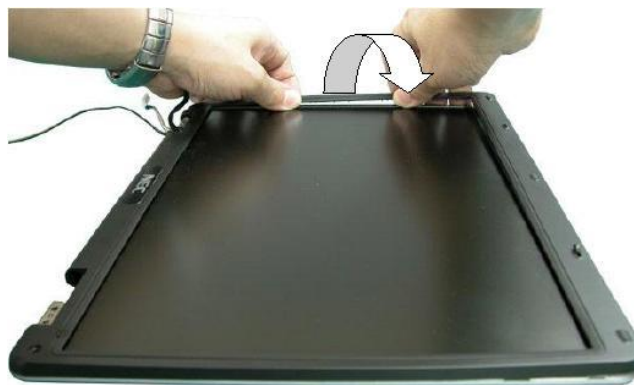
Fig. 19 Removing the LCD cover.
