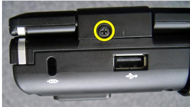
Fig. 10 Left keyboard back screw.
