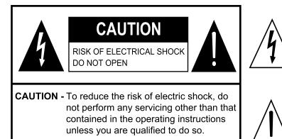
The lightning flash with arrowhead symbol, within an equilateral triangle is intended to alert the user to the presence of insinuated dangerous voltage within the product's enclosure that may be of sufficient magnitude to constitute a risk of electric shock to persons.
