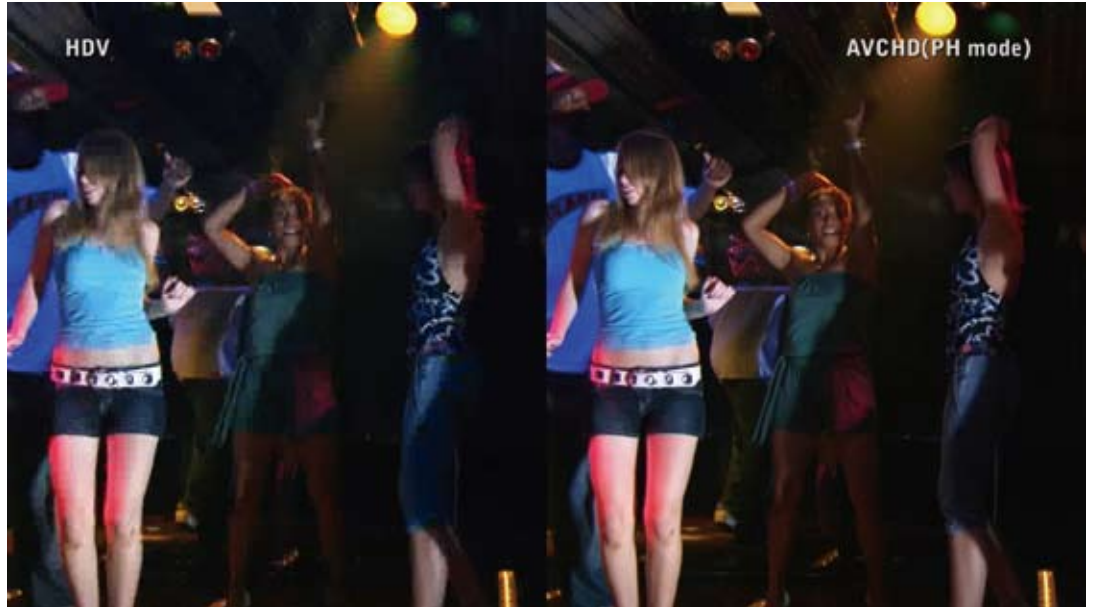
Sample comparison: When a flash causes large contrast differences and reduces depth perception, HDV shows considerable block noise, while AVCHD in the PH mode minimize break-up.
