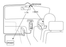
Take the following into account when installing the microphone and the antenna.
