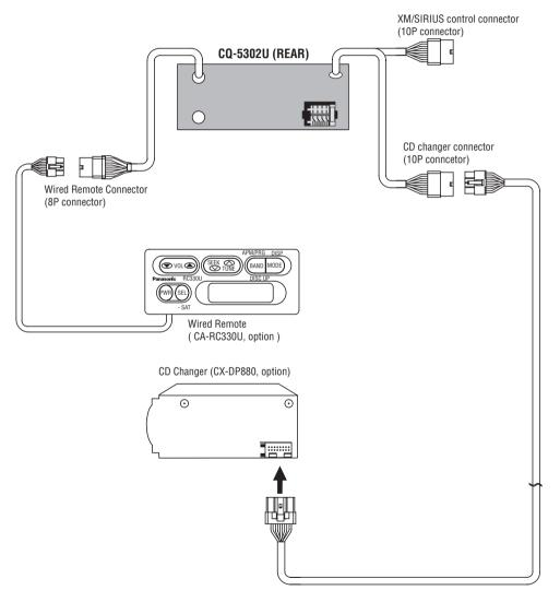
Extension Cable for connecting the unit and CD changer.
