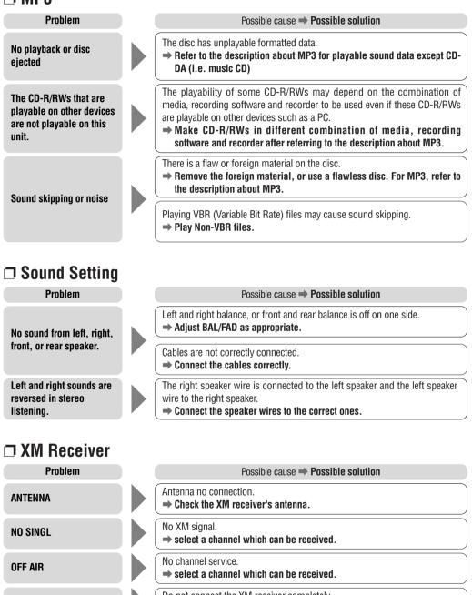
Do not connect the XM receiver completely. → Check the XM receiver's connections.
