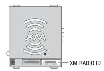
• Check the ID shown by tuning your XM Radio to channel 0. (Refer to "XM ID Confirmation" on page 25).
