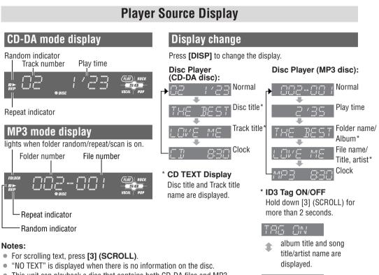
This unit can playback a disc that contains both CD-DA files and MP3 files. (Mixed Mode CD)
