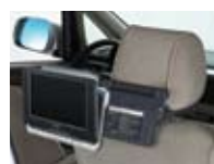
2 Mount the DVD-LS80 into the car bracket.
