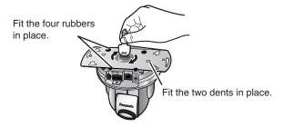
4 Attach the Ceiling Plate A to the Ceiling Plate B and attach them firmly with Screws A.
