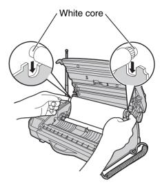
**5** If the ink film is slack, tighten it by winding the "T" shaped gear (blue).
