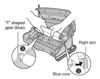
4 Insert the white core into the slots shown in the picture below.
