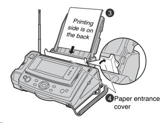
Install the recording paper cover on the recording paper tray by sliding it down from the top.
