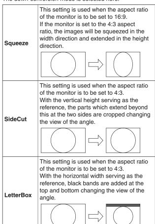
When output is selected for the color bar, the mode is fixed to Squeeze.
