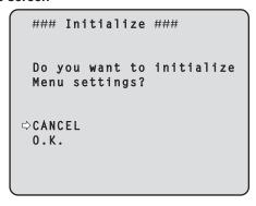
When the cursor is moved to "O.K." on the Initialize screen and the setting is entered, the Menu settings initialize screen is displayed for 5 seconds, and the camera settings are restored to the settings which were established when the camera was purchased.
