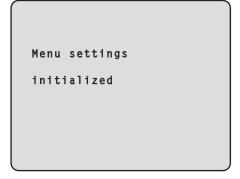
When the cursor is moved to "CANCEL" on the Initialize screen and the setting is entered, the Menu settings unchanged screen is displayed for 5 seconds, the initialization operation is not performed, and the Maintenance screen returns to the display.
