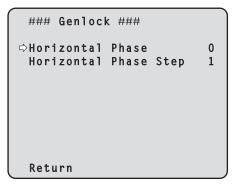
Press the [▲] or [▼] button to bring the cursor to "Horizontal Phase", and press the [○] button.
