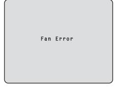
When the "Fan Error" message is displayed, request replacement of the cooling fan.
