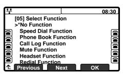
o If the selected function is Speed dial, enter the speed number and press the OK softkey. To enter alphanumeric characters select the Mode softkey. Refer to Appendix A for the character mapping of dial pad digits.
