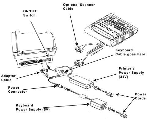
3. Attach the other end of the adaptor cable to the 9-pin port on the printer. Tighten the screws on the cables.
