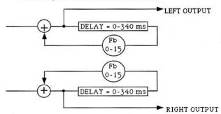
Stereo Multi-tap Echo: Up to 680 milliseconds of Delay Time in either of the left or right channel Taps. A single Feedback is taken from the Tap with the longer Delay Time. This Feedback is also programmable with up to 15 levels.
