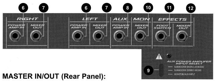
The MASTER IN/OUT section describes the functions related to the input and output patch panel located on the rear of your XR 1600F. This section is often overlooked but adds the most versatility to the XR 1600F. When used to its fullest potential, an extraordinary variety of wiring configurations can be made. These connections allow for devices such as outboard effects, additional power amps, monitors, and virtually any other type of line level audio device to be patched to the XR 1600F.
