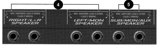
amplifier's speaker outputs. Both the LEFT/MON and RIGHT/L+R SPEAKER OUTPUTS provide two 1/4" jacks in parallel. By connecting a speaker cable(s) to this jack and to a speaker cabinet(s), you complete the signal chain. Several cabinets may be connected to each channel, as long as the combined impedance of the cabinets is not less than 4 ohms. (i.e., two 8 ohms cabinets in parallel = 4 ohms, four 16 ohms speakers in parallel = 4 ohms, etc.).
