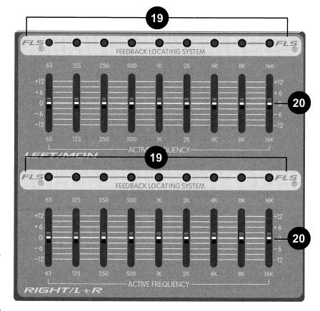
to decrease that frequency band's gain in order to lessen or eliminate feedback. (NOTE: These LEDs illuminate with any audio signal, not just during feedback.)
