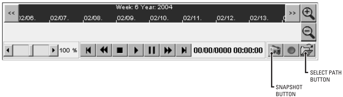
Figure 39. NVR-Playback Controls Used to Take a Snapshot
