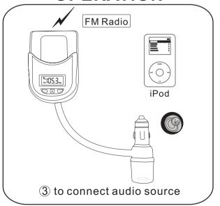
Adjust the frequency of car FM radio to the same frequency as transmitter for receicing signals. Free Manuals Download Website
