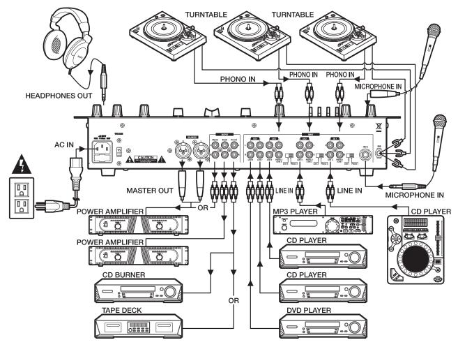
This mixer permits connection of up to ten (10) audio input sources, including two microphones. Such a system might include, for examples:
