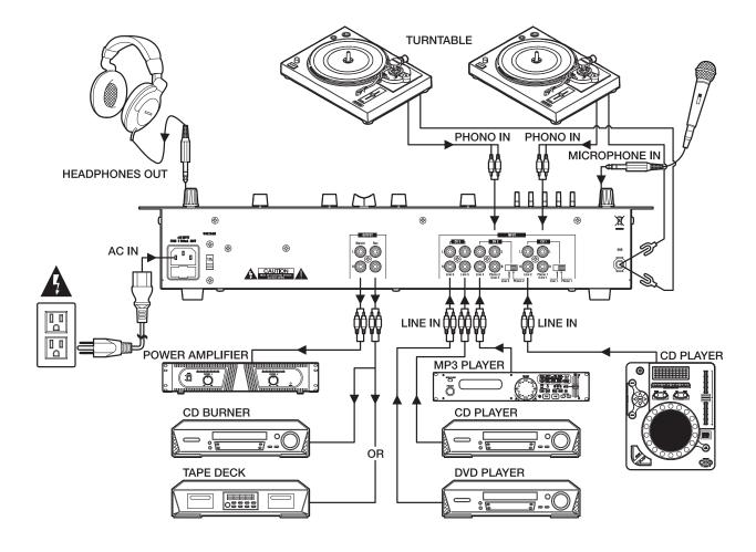
This mixer permits connection of up to seven (7) audio input sources, including one microphone. Such a system might include, for examples:
