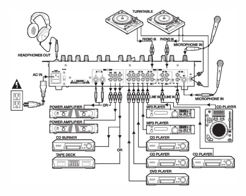
This mixer permits connection of up to eleven (11) audio input sources, including two microphones. Such a system might include, for examples:
