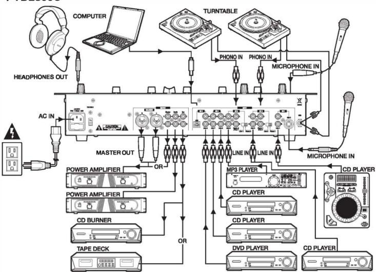
This mixer pennits connection of up to eleven (11) audio input sources, including two microphones. Such a system might include, for examples:
