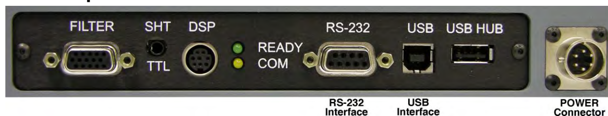
Figure 2-1. Details of the RS-232, USB, and Power Connections on the IsoPlane
