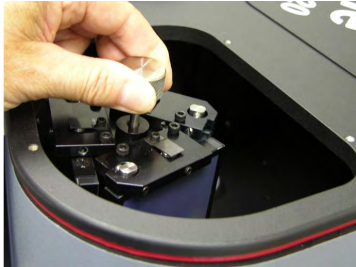
Figure 2-18. Lift Turret up out of the Turret Compartment
