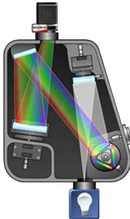
Figure 1-1. Light Path within the IsoPlane SCT 320
