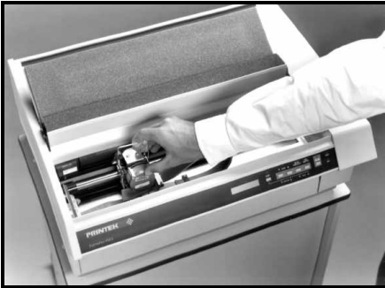
Lowering (closing) Ribbon Loading Bail
