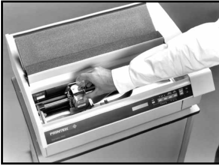
Closing the Ribbon Load Handle
