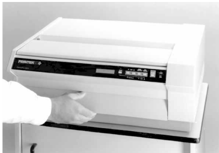
Opening The Latch Panel
