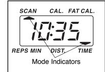
is selected, and a flashing mode indicator will show which mode is currently displayed. Note: If a different mode is selected, you can select the scan mode again by repeatedly pressing the mode button.
