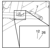
gap between the Reed Switch and the Magnet should be about 1/8". Make sure that the Magnet will not hit the Reed Switch when the Pedal Leg is moved. Repeat until the console displays correct feedback.
