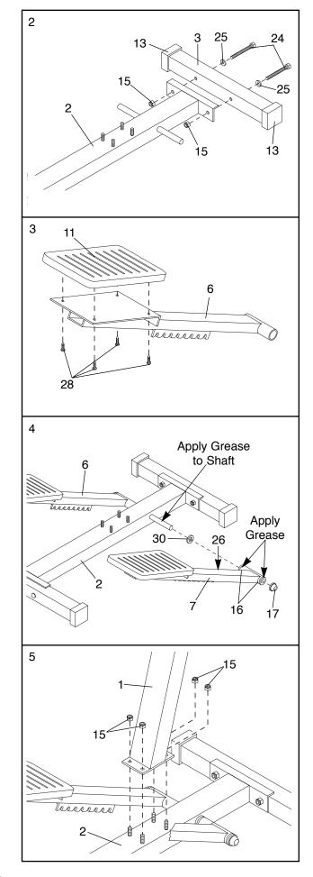
6. Apply grease to the shafts on the Upright (1).
