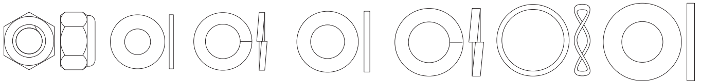
M8 Nylon Locknut (46)-4 M6 Washer (58)-2 M8 Split Washer (94)-10 M8.5 Washer (53)-2 M10 Split Washer (144)-2 Wave Washer (150)-2 M10 Washer (99)-2
