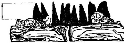
Figure 19 - Correct Flame Pattern with heater set to High Flame
