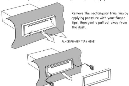
Insert the provided removal key into the opening on each side of the CD player. Push the keys inward until they snap in place. Firmly grab the keys and slowly pull the CD player out away from the dash.
