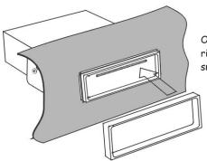
Once the CD player is secured, fit the trim ring over outside edge of the radio until it snaps into place.
