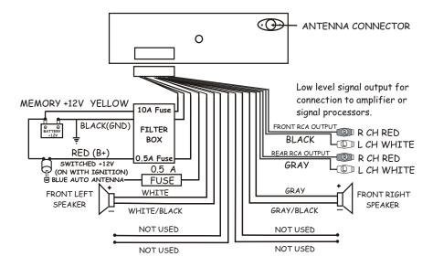
**CAUTION!** Tape unused wires so they do not short against other wires or chassis ground.
