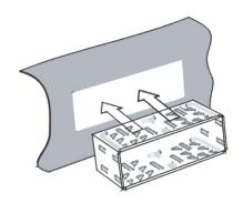
Insert the mounting sleeve into a standard DIN cutout in the dash kit, dashboard or Console.
