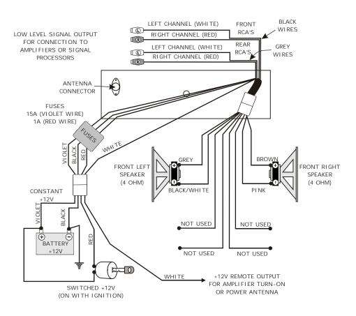
CAUTION! Tape unused wires so they do not short against other wires or chassis ground.
