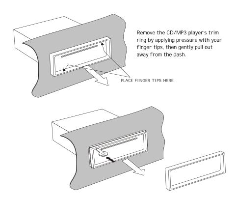
Insert the provided removal key into the opening on the top left side of the CD/MP3 player. Push the key inward until they snap into place. Firmly grab the key and slowly pull the CD/MP3 player out away from the dash.
