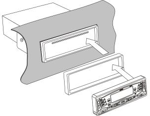
Once the CD/MP3 player is secured, fit the trim ring over outside edge of the radio until it snaps into place. I nsert the face plate with the right side first. Angle in the right side slightly then gently push the left side of face plate until it snaps completely in place.
