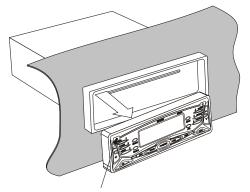
In order to remove the CD/MP3 player you will first need to release and detach the front panel.
