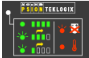
Figure 9.7 Battery Charge Status
