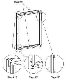
STEP 11 to bracket. Re-assemble door hinge bracket to previous position with bushing attached.
