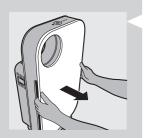
1 Place your fingers in the recesses of the side panels and gently pull the top part of the front panel towards you. Then lift the hooks at the bottom of the panel out of the bottom of the appliance.
