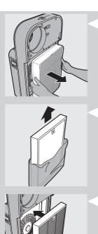
2 Remove the filters from the appliance.
