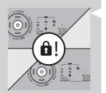
If you do not replace the filter in time, the appliance stops operating approx. 2 weeks after the filter replacement light started flashing. When the appliance is locked, it does not operate until you have replaced with the new filter and pressed the reset button.
