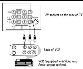
You can view the playback of VCR tapes (Video Disc players, camcorders, etc.) by using the AUDIO and VIDEO INPUT sockets on the rear of the TV.
