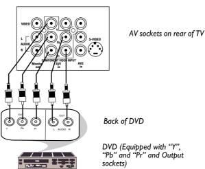
You can view the playback of DVD discs by using the COMPONENT VIDEO INPUT sockets on the rear of the TV.
