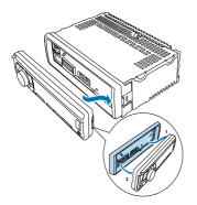
**3** Press the left side of the panel until it is locked into place.
