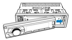
2 Press the left end of the front panel inwards until it is securely locked with a "click".
