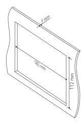
• Since the unit cannot be used if the dashboard opening's slant angle is above 20 degrees, make sure that the horizontal slant of the car dashboard opening is between 0 and 20 degrees.
