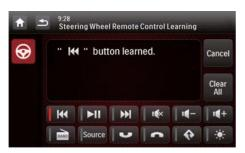
5 Repeat steps 3 and 4 to assign more functions to buttons on the steering wheel.
