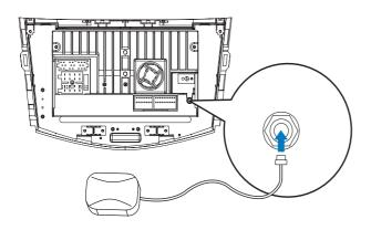
2 Stick the other end of the GPS antenna to a surface for signal reception.
