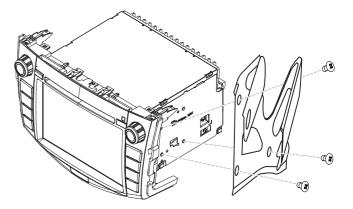
4 Fix the unit to the dashboard with screws (supplied by the car manufacturer).
