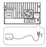
2 Stick the other end of the GPS antenna to a metal surface of the car.
