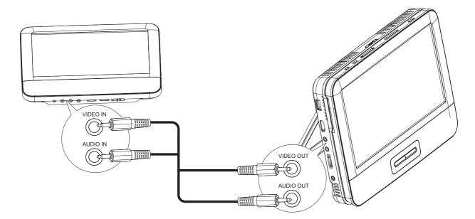
Connect the supplied AV cable to:
