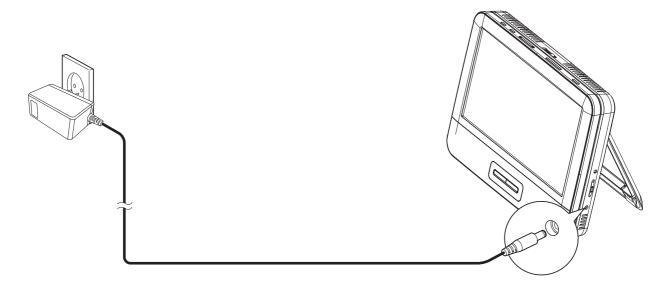
1 Connect the AC adaptor to the **DC IN** jack on the main unit and the power outlet.
