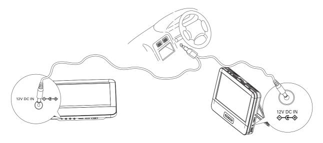
1 Connect the car adaptor to the **DC IN** jack on the main unit and the second screen first, then connect it to the car cigarette lighter socket.
