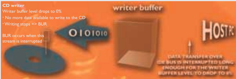
Fig. 3, Typical CD writing process: Buffer under run occurs and results in writing failure, disc is ruined.
