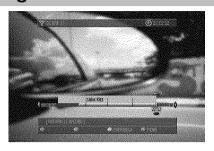
As soon as you turn on the DVD recorder, the currently selected TV channel on the DVD-Recorder is recorded in a temporary storage (Time shift Buffer).
