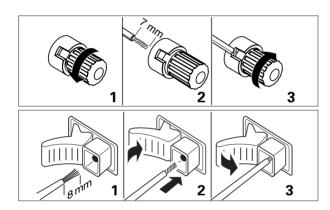
1 Always connect the coloured (or marked) wire to the coloured terminal and the black (or unmarked) wire to the black terminal.
