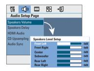
Use ◀ ► keys to set the volume level for each speaker (-6dB ~ +6dB) and press OK to confirm.
