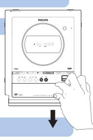
**IMPORTANT!** Slide down to expose some buttons and jacks on the front panel!
