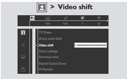
Press ◀▶ to adjust the horizontal position of the picture on your TV screen by scrolling the slider to the left or right.
