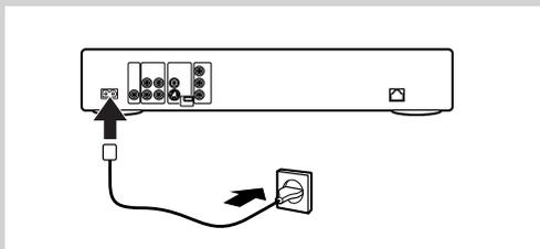
**5 Connect the mains cable between the AC Mains input ⑨ of the SL400i and a mains socket.**
