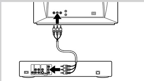
**4 Connect the Audio + Composite video cable to the audio and video outputs ⑮ of the SL400i and to your TV.**
