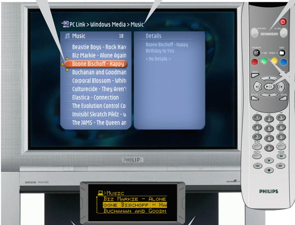
*Option: If menu choices are displayed in the lower left and lower right corner of the LCD, use the buttons on the SL400i on either side of the LCD to enter your choice.*
