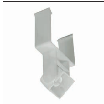
The ZTX400 MB-MDU is a Linesense mounting bracket for clicking movement detector LRM 8115/00 or LRM 8117/00 to the trunking section. The right tilt angle can be adjusted manually and is to be checked by a walk test. The same tilt angle can be easily reproduced on more sensors thanks to a click graduation on the bracket
